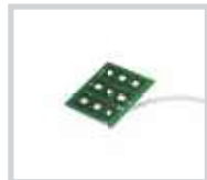
EVA.LAMP Circuit for flashing light.
