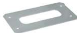
Foundation plate with anchor bolts included. Motor and floor fixing distance 269x106 mm, no. 4 Ø 12 mm.
